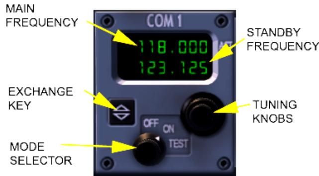
Figura 6.9.1. Panel COM auxiliar
